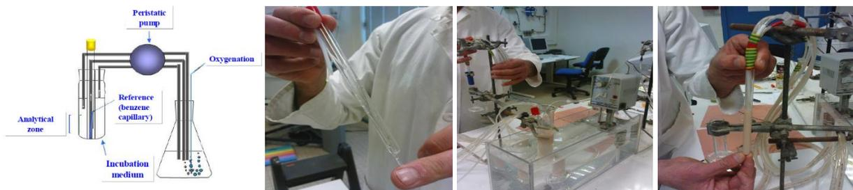
Fig. 1 Perfusion system for *in vivo* NMR described by Choraio et al. 2009.
