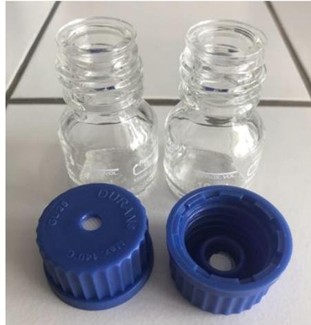
**Figure 7** Vials with sterile-venting membrane screw caps.
