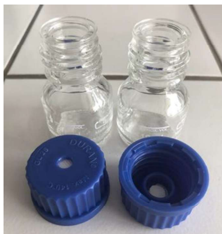
Figure 7 Vials with sterile-venting membrane screw caps.
