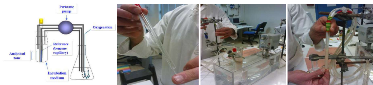
Fig. 1 Perfusion system for in vivo NMR described by Choraó et al. 2009.
